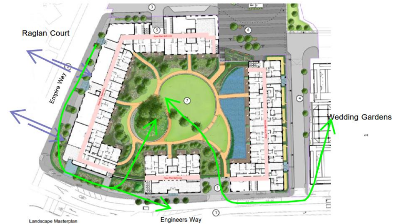
The overall planting arrangement allows a natural corridor for fauna to navigate in around the development and provides a link to the gardens at Brent Civic Centre and Raglan Court
