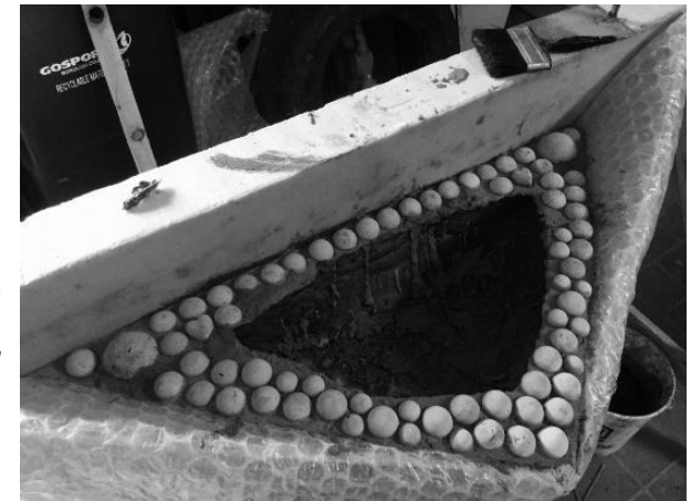
One of the Fishbourne artificial rockpools (Vertipools) in the mould:
