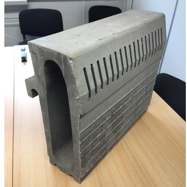
Kerb specially designed to prevent lizards and toads from entering the drainage system:
