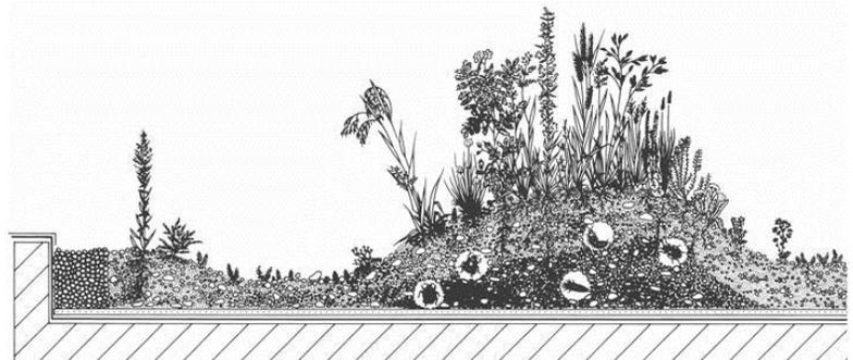
*Photo: Biodiverse green roof cross section*
