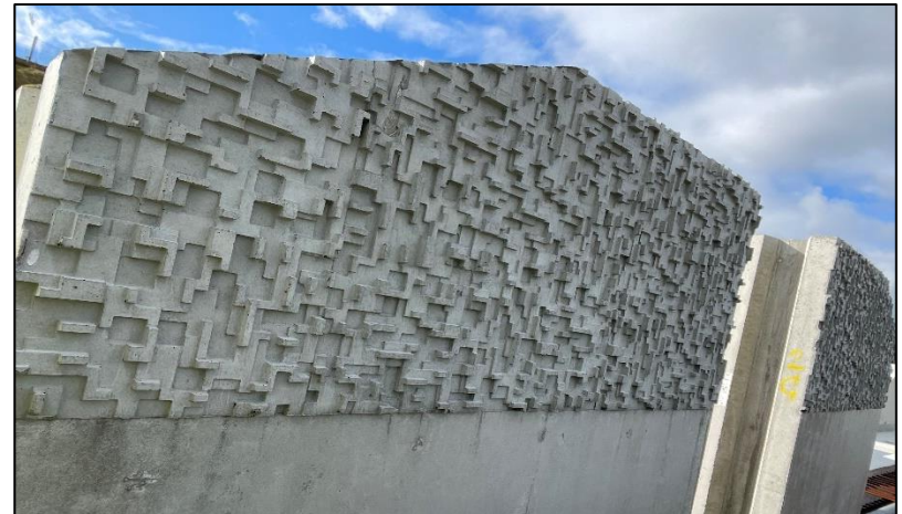
Banagher Precast Concrete produced precast seawall units with ECO Seawall surface finish, achieved using the ECO seawall formliner with Azouri pattern (ECONcrete®) – Conwy County Borough Council
